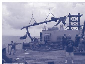
John Broadwater watches as the rudder support skeg is lowered on deck.
