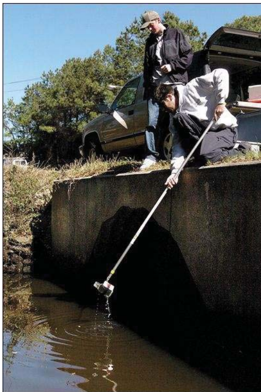
Brad Rosov (right), a technician with the UNCW Center for Marine Science Research, takes a sample Monday from Hewletts Creek where it passes under Pine Grove Drive. He and student Asher Williams were testing for effects of sewage spills.
