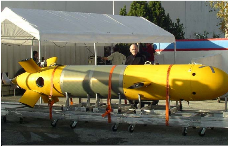
Explorer-Class Deepwater AUV completing factory acceptance testing at ISE.
