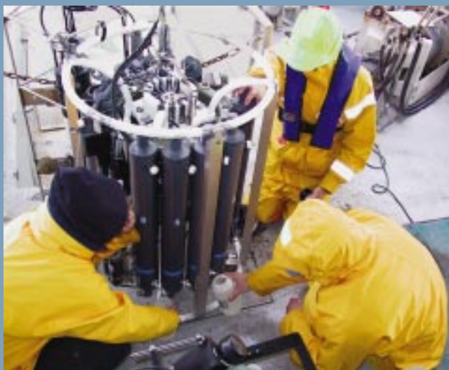
Students from the Cruise or Field Sampling course work together to remove water samples taken via a carousel water sampler that is used by researchers to help determine the health of the coastal ocean ecosystem. The students enrolled in this course participate in the planning and sampling phases of major marine or environmental research programs.
